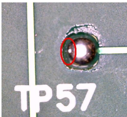
Test Point 57 After (with witness mark)
